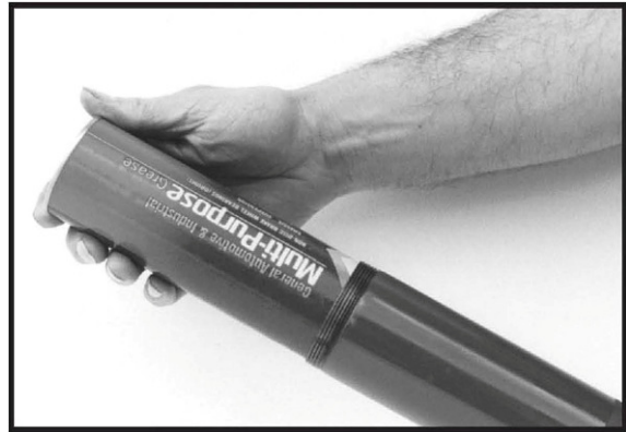
Installing Grease Cartridge
